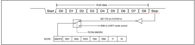
Figure 15–7. UART0 Frame Error Detection
