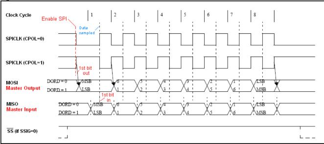
Figure 18-7. SPI Master Transfer Format with CPHA=0
