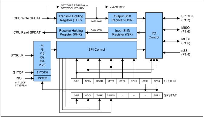
Figure 18–1. SPI Block Diagram
