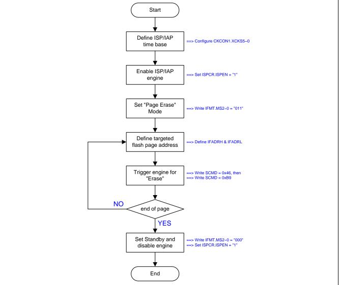
Figure 22–3 shows the demo code of the ISP/IAP page erase operation.
