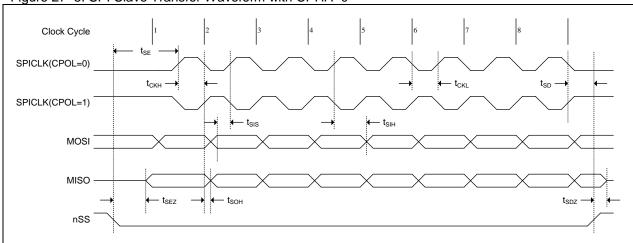
Figure 27-5. SPI Slave Transfer Waveform with CPHA=0
