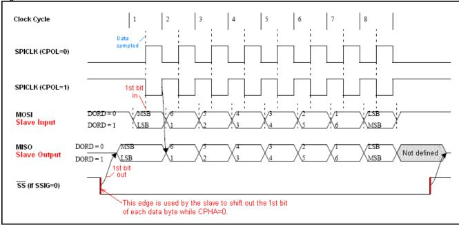
Figure 18–5. SPI Slave Transfer Format with CPHA=0
