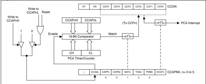
Figure 17–5. PCA Software Timer Mode
