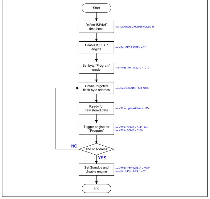
Figure 22–5 shows the demo code of the ISP/IAP byte program operation.
