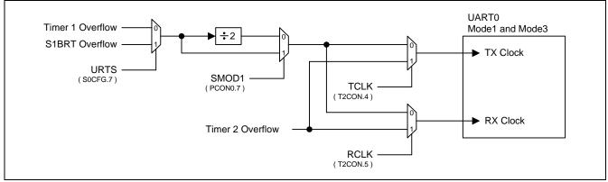
Figure 16-4. Additional Baud Rate Source for the UART0
