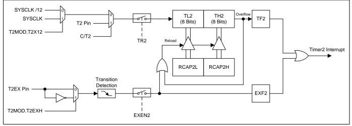
Figure 14–7. Timer 2 in Auto-Reload Mode (DCEN=0)
