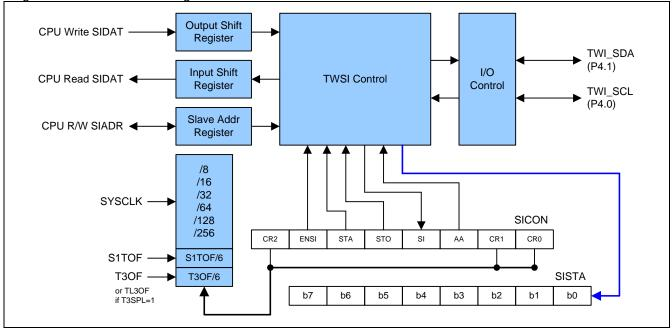
Figure 19-2. TWSI Block Diagram
