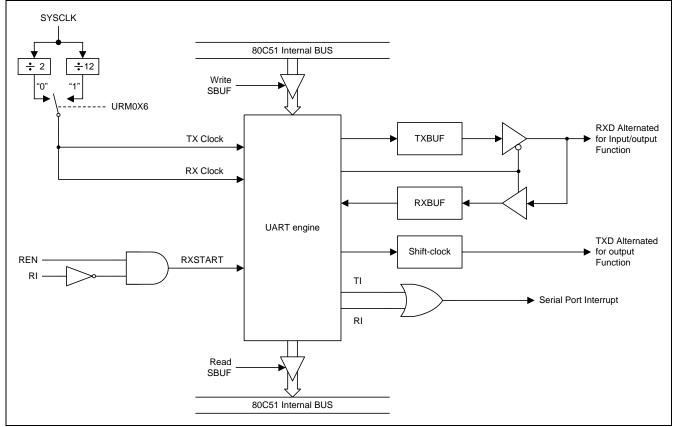
Figure 15-3. Serial Port 0 Mode 0
