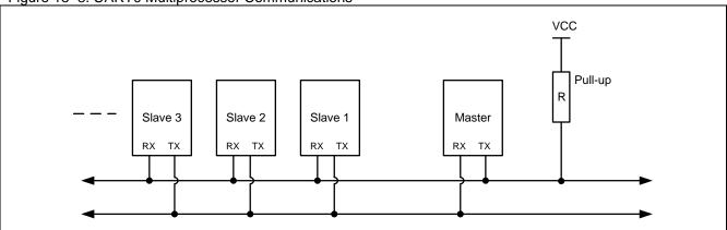
Figure 15-8. UARTO Multiprocessor Communications
