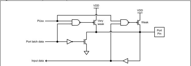
Figure 12-5. General Open-Drain Output
