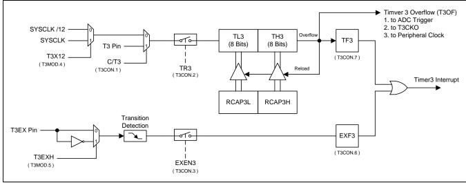
Figure 14-11. Timer 3 in 16 bit Auto-Reload Mode (T3SPL=0)
