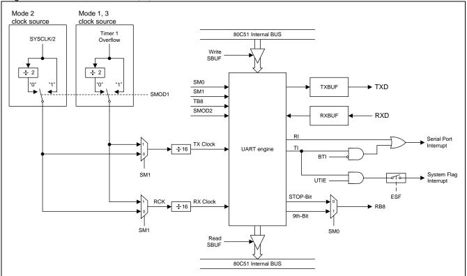
Figure 15-6. Serial Port Mode 1, 2, 3
