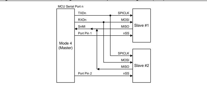
The SPI master satisfies the transfer with the full function SPI module of Megawin MG82/84 series MCU with CPOL, CPHA and DORD selection. For CPOL and CPHA condition, **MG82FG5BXX** uses an easy way by initialize SPI clock assigned port pin (TXD1, P1.3/P3.4) polarity to fit them. Table 18–6 shows the serial port Mode 4 mapping with the four SPI operating mode.
