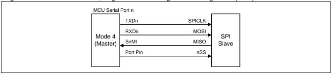
Figure 18–3. Serial Port Mode 4, Single Master and Multiple Slaves configuration (n = 1)
