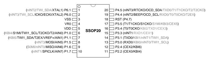
Figure 5-5. MG82FG5BxxAL16 Top View
