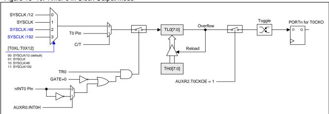
Figure 16-11. Timer 1 in Clock Output Mode
