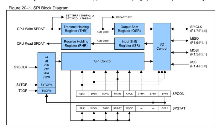
The SPI interface has four pins: MISO (P1.6), MOSI (P1.5), SPICLK (P1.7) and nSS (P1.4):
