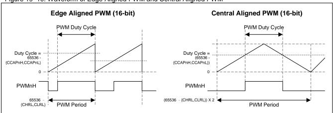
Bit 6: EXDT: Extend Dead-Time in PWM Period. This enabled function will corrupt the non-PWM channel function. Such as capture mode, software timer mode and high speed output mode. The waveform of EXDT control bit is show in Figure 1-7.
