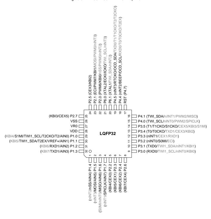
Figure 5-2. MG82FG5BXXAY32 Top View
