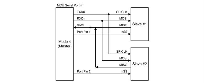
The SPI master satisfies the transfer with the full function SPI module of Megawin MG82/84 series MCU with CPOL, CPHA and DORD selection. For CPOL and CPHA condition, **MG82FG5BXX** uses an easy way by initialize SPI clock assigned port pin (TXD0, P3.1/P4.5) polarity to fit them. Table 17–21 shows the serial port Mode 4 mapping with the four SPI operating mode.
