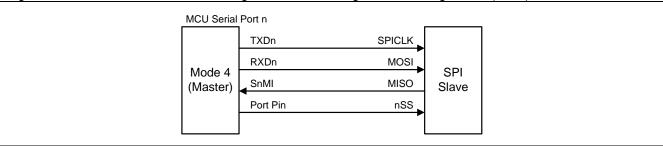
Figure 17–11. Serial Port 0 Mode 4, Single Master and Multiple Slaves configuration (n = 0)
