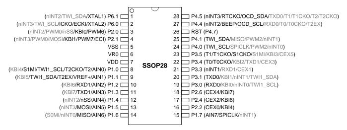
Figure 5-4. MG82FG5BxxAL20 Top View
