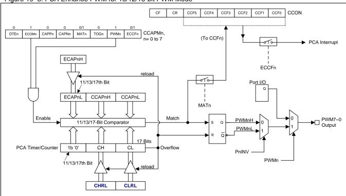
Figure 19–9. PCA Enhance PWM for Buffer Mode (PWM6/7 have no dead-time control function)
