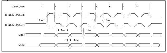
Figure 31–4. SPI Master Transfer Waveform with CPHA=1
