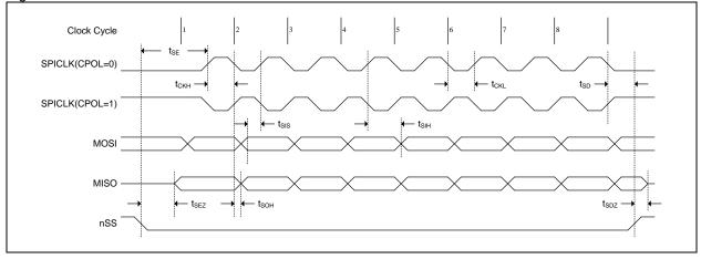
Figure 31-6. SPI Slave Transfer Waveform with CPHA=1
