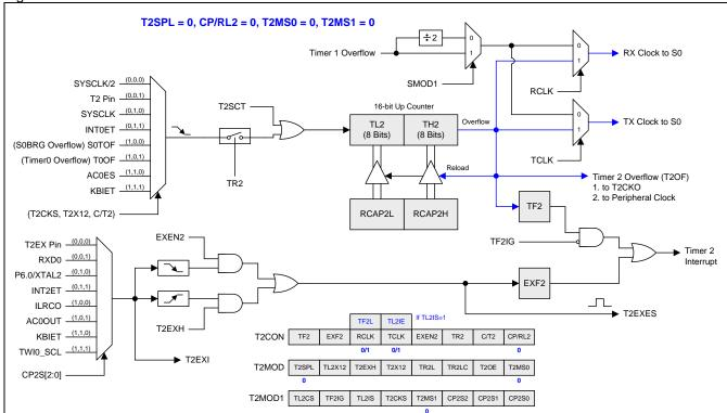
Figure 15-21. Timer 2 in Baud-Rate Generator Mode
