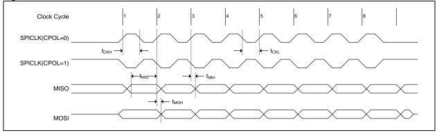
Figure 31-5. SPI Slave Transfer Waveform with CPHA=0
