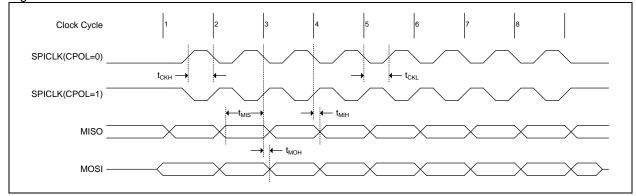
Figure 31-4. SPI Master Transfer Waveform with CPHA=1
