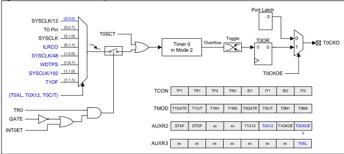
Figure 15-11. Timer 1 in Clock Output Mode
