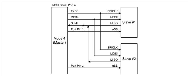
The SPI master satisfies the transfer with the full function SPI module of Megawin MG82/84 series MCU with CPOL, CPHA and DORD selection. For CPOL and CPHA condition, **MG82FG5D16** uses an easy way by initialize SPI clock polarity to fit them. Table 17–37 shows the serial port Mode 4 mapping with the four SPI operating mode.
