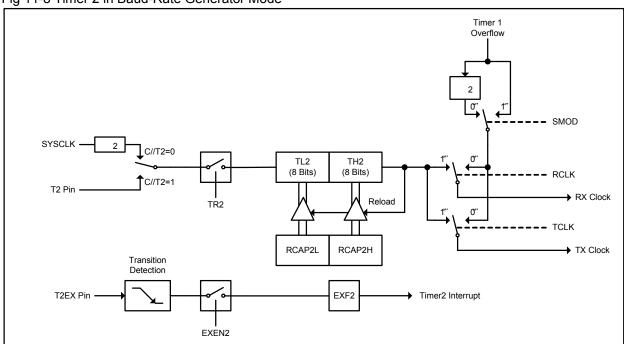
Fig 11-8 Timer 2 in Baud-Rate Generator Mode
