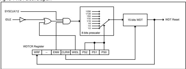
To enable the WDT, users must set ENW bit (WDTCR.5). When the WDT is enabled, the counter will increment one by an interval of (12 x Prescaler / SYSCLK). And now the user needs to clear it by writing "1" to the CLRW bit (WDTCR.4) before WDT overflows. When WDT overflows, the CPU will reset itself and re-start.
