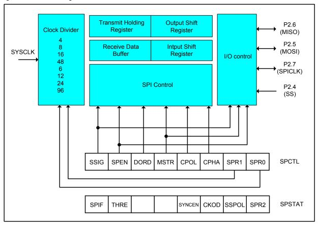
The SPI interface has four pins: MISO (P2.6), MOSI (P2.5), SPICLK (P2.7) and /SS (P2.4):
