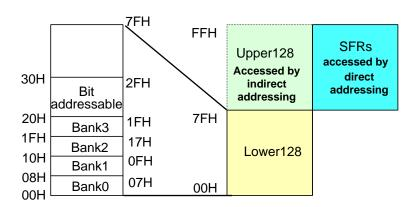
MG87FE/L04 has internal data RAM that is mapped into three separate segments. They are lower 128 bytes of RAM, upper 128 bytes of RAM and 128 bytes Special Function Register (SFR).
