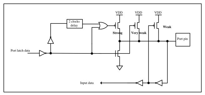
By the way, the pull-up resistor is disabled on P10/P11 in default.
