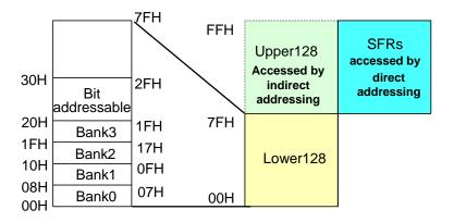
MG87FE/L2051/4051/6051 has internal data RAM that is mapped into three separate segments. They are lower 128 bytes of RAM, upper 128 bytes of RAM and 128 bytes Special Function Register (SFR).
