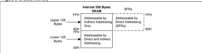
Figure 6-3. Lower 128 Bytes of Internal RAM
