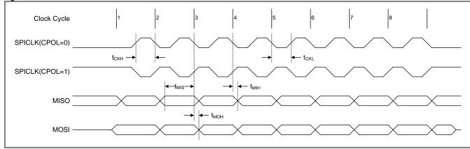
Figure 23-4. SPI Master Transfer Waveform with CPHA=1
