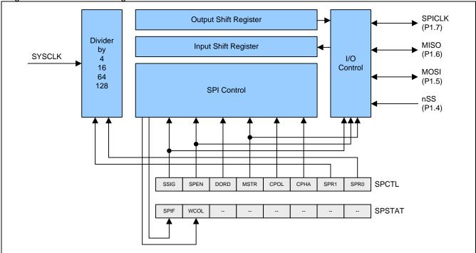
The SPI interface has four pins: MISO (P1.6), MOSI (P1.5), SPICLK (P1.7) and nSS (P1.4):
