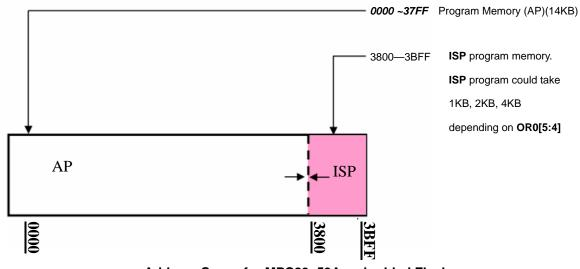
Address Space for MPC89x53A embedded Flash memory
