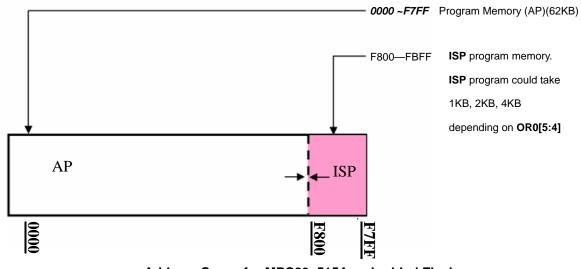
Address Space for MPC89x515A embedded Flash memory
