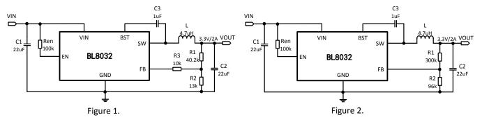
**Note:** 1) C1 and C2 recommended using 22uF ceramic capacitors. If the electrolytic capacitor is used, it is recommended that the ceramic capacitor in parallel with a capacitance value of 0.1uF or more.
