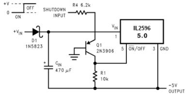
Figure 9. Inverting Regulator Ground Referenced Shutdown
