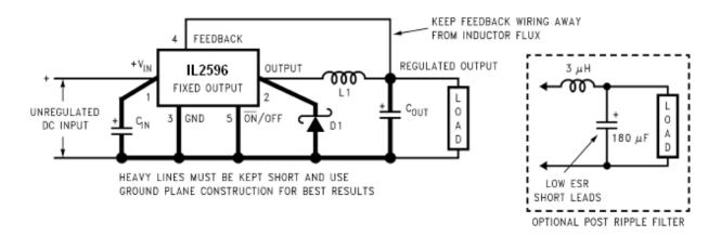
CIN —470  $\mu$ F, 50V, Aluminum Electrolytic Nichicon "PL Series" COUT —220  $\mu$ F, 25V Aluminum Electrolytic, Nichicon "PL Series" D1 —5A, 40V Schottky Rectifier, 1N5825 L1 —68  $\mu$ H, L38
