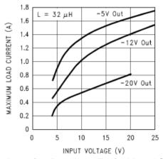
Figure 8. Inverting Regulator Typical Load Current
