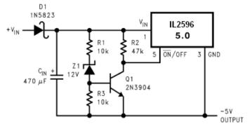
This circuit has hysteresis Regulator starts switching at VIN = 13V Regulator stops switching at VIN = 8V
