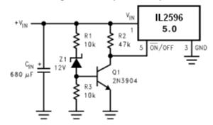
Figure 4. Undervoltage Lockout for Buck Regulator
