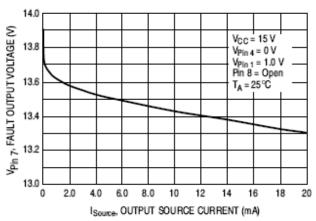
Figure 25. Fault Output High State Voltage versus Source Current
