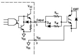
Figure 32. Using Separate Resistors for Turn-On and Turn-Off
