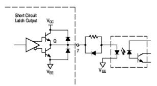
Figure 33. Output Fault Optoisolator
