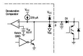
Figure 34. Desaturation Detection
