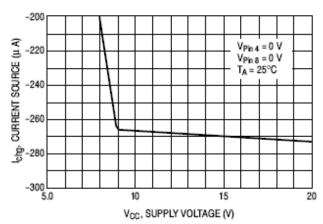
Figure 21. Fault Blanking/Desaturation Current Source versus Supply Voltage
