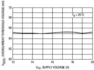
Figure 13. Overcurrent Protection Threshold Voltage versus Supply Voltage
