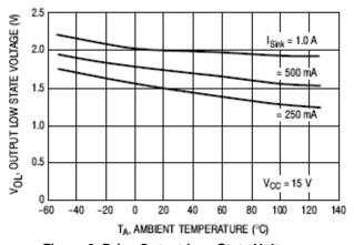
Figure 6. Drive Output Low State Voltage versus Temperature
