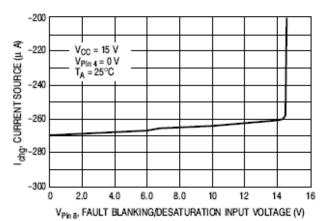
Figure 22. Fault Blanking/Desaturation Current Source versus Input Voltage
