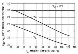
Figure 4. Input Threshold Voltage versus Temperature
