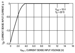
Figure 16. Current Sense Input Current versus Voltage
