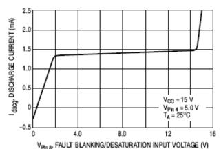
Figure 23. Fault Blanking/Desaturation Discharge Current versus Input Voltage
