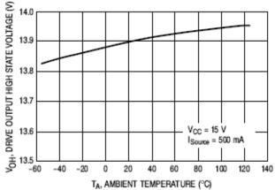
Figure 8. Drive Output High State Voltage versus Temperature
