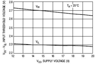
Figure 5. Input Threshold Voltage versus Supply Voltage
