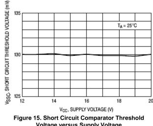
Voltage versus Supply Voltage
