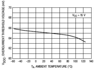
Figure 12. Overcurrent Protection Threshold Voltage versus Temperature
