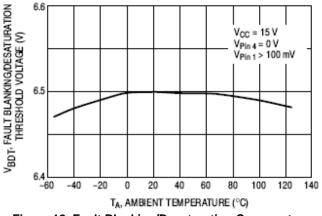
Figure 18. Fault Blanking/Desaturation Comparator Threshold Voltage versus Temperature
