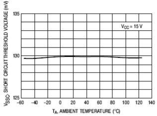
Figure 14. Short Circuit Comparator Threshold Voltage versus Temperature
