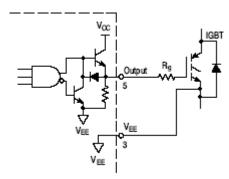
Figure 31. Using a Single Gate Resistor
