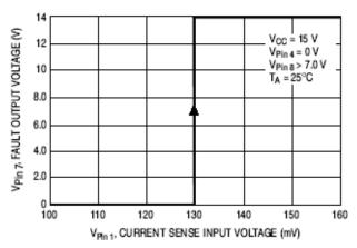
Figure 11. Fault Output Voltage versus Current Sense Input Voltage
