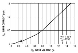
Figure 2. Input Current versus Input Voltage
