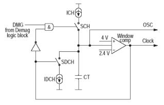
Figure 5. Oscillator Block
