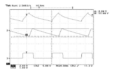
Figure 11. SMPS Pulsed Mode
