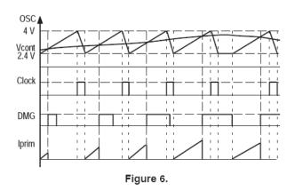
The OSC and Clock signals are provided according to the Figure 6. The Clock signals correspond to the CT capacitor discharge. The bottom curve represents the current flowing in the sense resistor Rcs. It starts from zero and stops when the sawtooth value is equal to the control voltage Vcont. In this way the SMPS is regulated with a voltage mode control.
