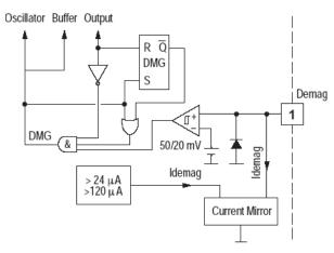
Figure 4. Demagnetization Block
