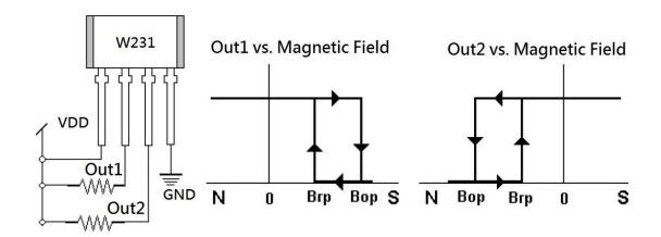
When Out1 and Out2 are short, W231 becomes Omnipolar Hall Effect Switch IC.
