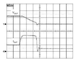
$C_{OUT}$ =10 $\mu$ F,  $C_{IN}$ =10 $\mu$ F,  $I_{OUT}$ =1A to 2.3A
