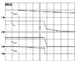
$$\begin{split} & C_{\text{OUT}} \! = \! 10 \mu \text{F}, \, C_{\text{IN}} \! = \! 10 \mu \text{F}, \, R_{\text{L}} \! = \! 1.2 \Omega \\ & \text{CH1: V}_{\text{CNTL}}, \, 5 \text{V/Div, DC} \\ & \text{CH2: V}_{\text{IN}}, \, 1 \text{V/Div, DC} \\ & \text{CH3: V}_{\text{OUT}}, \, 1 \text{V/Div, DC} \\ & \text{CH4: V}_{\text{POK}}, \, 5 \text{V/Div, DC} \\ & \text{TIME: 10ms/Div} \end{split}$$
