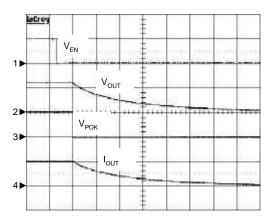
$C_{OUT} = 10\mu F, C_{IN} = 10\mu F, R_L = 1.2\Omega$ CH1:  $V_{EN}$ , 5V/Div, DC
