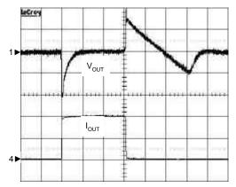
$I_{\text{OUT}} \text{=} 10 \text{mA}$  to 1A to 10mA (rise / fall time = 1  $\mu \text{s})$
