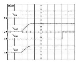
$\begin{array}{l} C_{\text{OUT}} \! = \! 10 \mu \text{F}, \, C_{\text{IN}} \! = \! 10 \mu \text{F}, \, R_{\text{L}} \! = \! 1.2 \Omega \\ \text{CH1: V}_{\text{EN'}}, \, 5 \text{V/Div, DC} \\ \text{CH2: V}_{\text{OUT'}}, \, 1 \text{V/Div, DC} \\ \text{CH3: V}_{\text{POK'}}, \, 5 \text{V/Div, DC} \\ \text{CH4: I}_{\text{OUT'}}, \, 1.0 \text{A/Div, DC} \\ \text{TIME: 0.5 ms/Div} \end{array}$
