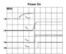
$\begin{array}{l} C_{OUT} \! = \! 10 \mu F, \, C_{IN} \! = \! 10 \mu F, \, R_L \! = \! 1.2 \Omega \\ CH1: \, V_{CNTL}, \, 5V/Div, \, DC \\ CH2: \, V_{IN}, \, 1V/Div, \, DC \\ CH3: \, V_{OUT}, \, 1V/Div, \, DC \\ CH4: \, V_{POK}, \, 5V/Div, \, DC \\ TIME: \, 5ms/Div \end{array}$
