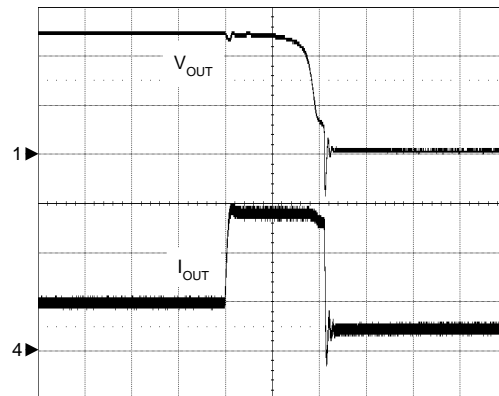
Over Current Protection
