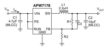
R1  $\leq$  1M $\Omega$  is recommended R2  $\leq$  200K $\Omega$  is recommended
