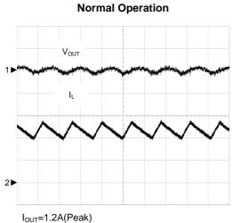
CH1: V<sub>OUT</sub>, 20mV/Div, DC offset 1.2V CH2: I<sub>L</sub>, 0.5A/Div, DC TIME: 500ns/Div
