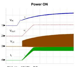
CH1: VIN, 10V/Div, DC CH2: Vout, 2V/Div, DC CH3: VLx, 10V/Div, DC CH4: IL, 5A/Div, DC TIME: 1ms/Div
