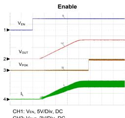
CH1: Ven, 5V/Div, DC CH2: Vout, 2V/Div, DC CH3: Vpok, 5V/Div, DC CH4: IL, 5A/Div, DC TIME: 500μs/Div
