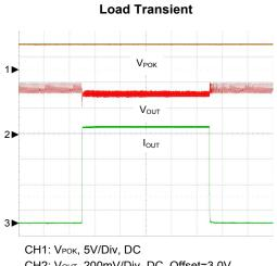
CH1: VPok, SV/Div, DC CH2: Vout, 200mV/Div, DC, Offset=3.0V CH3: Iout, 2A/Div, DC TIME: 1ms/Div
