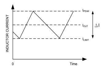
Figure 1. Current Limit algorithm
