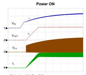
CH1: VIN, 10V/Div, DC CH2: VOUT, 2V/Div, DC CH3: VLX, 10V/Div, DC CH4: IL, 5A/Div, DC TIME: 1ms/Div
