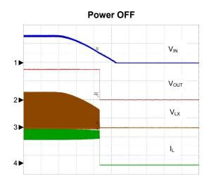
CH1: V<sub>IN</sub>, 10V/Div, DC CH2: V<sub>OUT</sub>, 2V/Div, DC CH3: V<sub>LX</sub>, 10V/Div, DC CH4: I<sub>L</sub>, 5A/Div, DC TIME: 2ms/Div
