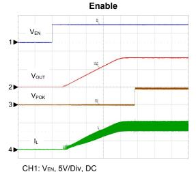
CH2: Vout, 2V/Div, DC CH3: Vpok, 5V/Div, DC CH4: IL, 5A/Div, DC TIME: 500µs/Div
