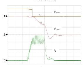
CH1: VPOK, 5V/Div, DC CH2: VOUT, 2V/Div, DC CH3: IL, 5A/Div, DC TIME: 20µs/Div
