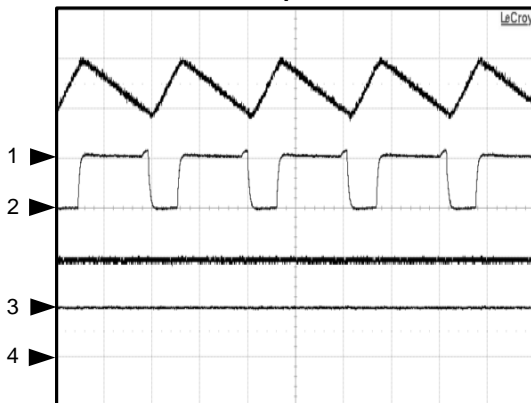
Boost Mode, V_{BAT}=3.8V , I_{VBUS}= 500mA , In CCM Operation
