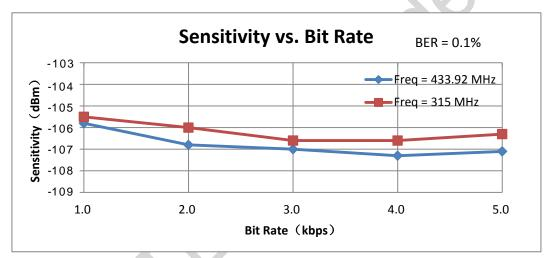
Figure 7. Sensitivity vs. Bit Rate
