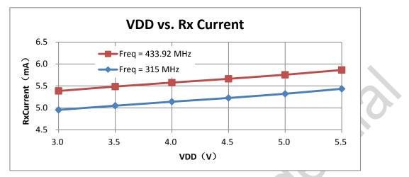
Figure 3. Rx Current vs. VDD
