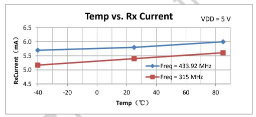
Figure 4. Rx Current vs. Operating Temperature
