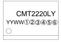
Figure 10. CMT2220LY Top Marking
