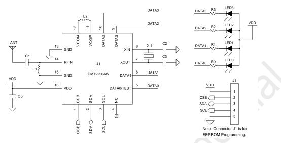
Figure 1. CMT2250AW Typical Application Schematic
