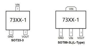
NOTE: XX indicate Output Voltage, xx indicate Data Code For example: 7333-1(Vout=3.3V)
