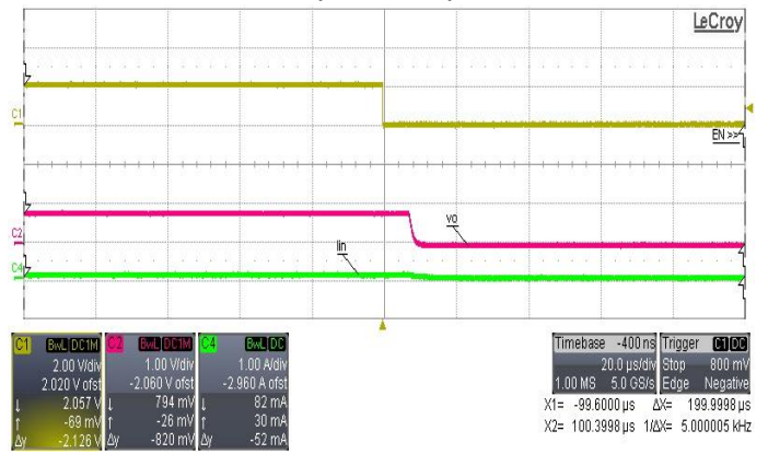
Turn off TOFF from VON, VIN=0.8V, VBIAS=5V CH1:VON, CH2:VO, CH3:IIN
