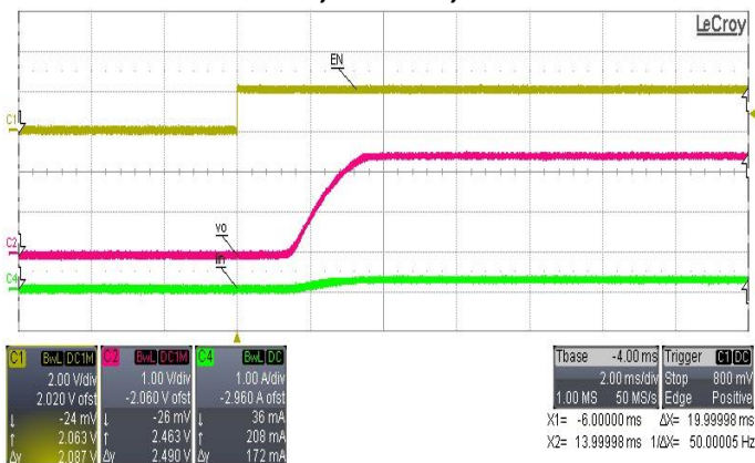
Von to Vo Ready, VIN=2.5V, VBIAS=2.5V. CH1:VON, CH2:VO, CH3:IIN
