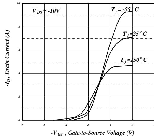
**Fig 12. Transfer Characteristics**
