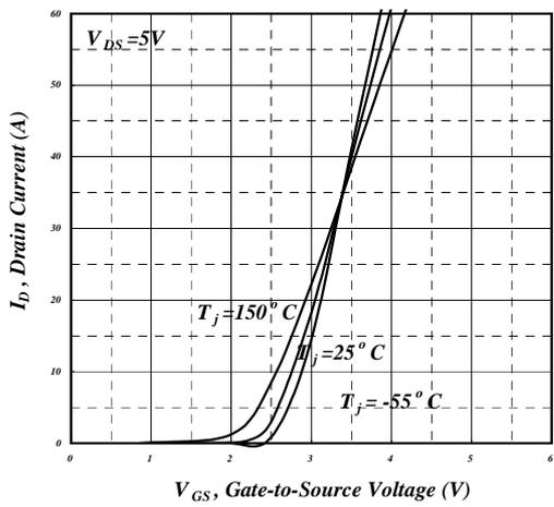
Fig 15. Transfer Characteristics
