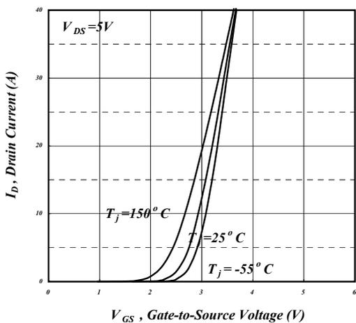
Fig 11. Transfer Characteristics
