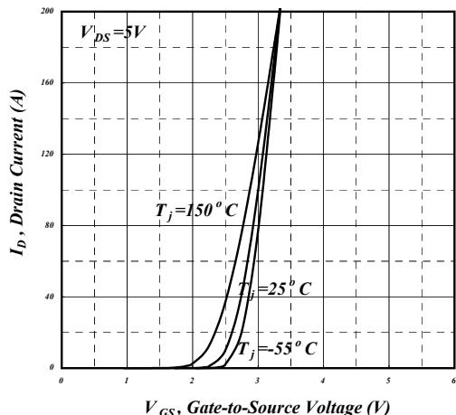
Fig 12. Transfer Characteristics
