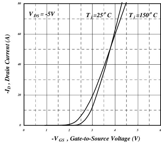
**Fig 14. Transfer Characteristics**
