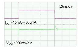
$\begin{array}{l} XC9267C75Cxx, \ f_{OSC}=1.2MHz \\ V_{\text{IN}}=16V \rightarrow 32V, \ V_{\text{OUT}}=3.3V, \ I_{\text{OUT}}=300\text{mA} \\ \text{L}=4.7\mu\text{H}(\text{CLF5030NIT-4R7}), \ C_{\text{IN}}=4.7\mu\text{F}\times2(\text{C2012X6S1H475K}) \\ C_{\text{L}}=10\mu\text{F}\times2 \ (\text{C3216X7R1E106K}) \end{array}$
