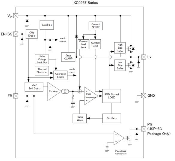
Diodes inside the circuit are an ESD protection diodes and a parasitic diodes.
