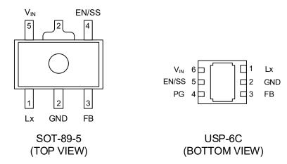
\* The dissipation pad for the USP-6C package should be solder-plated in recommended mount pattern and metal masking so as to enhance mounting strength and heat release. If the pad needs to be connected to other pins, it should be connected to the GND (No. 2) pin.
