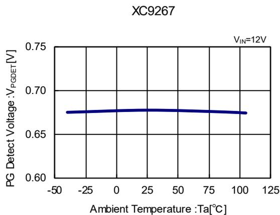
(13) PG Output Voltage vs. Ambient Temperature
