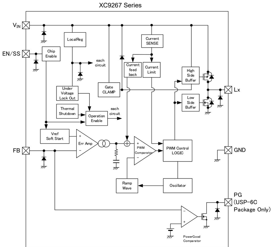
\* Diodes inside the circuits are ESD protection diodes and parasitic diodes.
