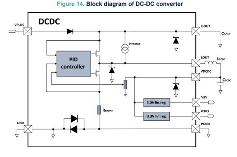
This block also includes a sense resistor (R<sub>SHUNT</sub>) to measure the inductor current, a series diode to prevent conduction during reverse polarization, and protection diodes to conduct residual inductor currents whenever switching ceases.
