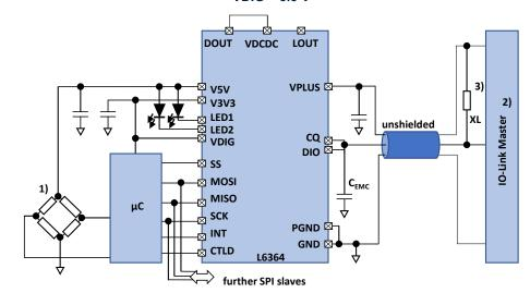
Figure 21. Application example: DC-DC disabled, CQ and DIO coupled (Join Mode), V<sub>SENSOR</sub> = 5 V, V<sub>MCU</sub> = VDIG = 3.3 V
