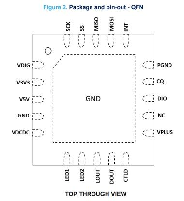
N.B. GND pin and Exposed pad to be shorted on PCB
