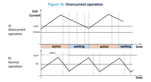
For coil protection purposes, the maximum duty is further limited by the L6364 in relation to the supply voltage so that the maximum coil current rise in one cycle is limited to:
