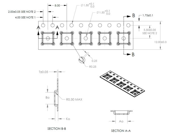
Note: 1: 10 SPROCKET HOLE PITCH CUMULATIVE TOLERANCE ±0.2 2: POCKET POSITION RELATIVE TO SPROCKET HOLE MEASURED AS TRUE POSITION OF POCKET, NOTPOCKET HOLE.
