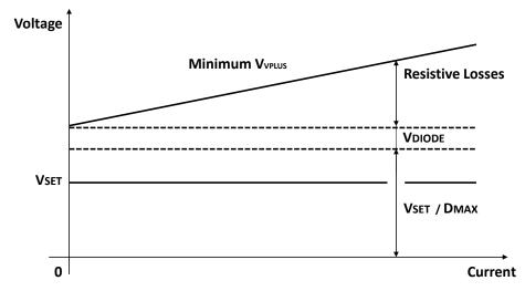
The supply voltage (V<sub>VPLUS</sub>) required to reach a nominal output voltage (V<sub>SET</sub>) is given by:  $V_{VPLUS} = V_{SET} / D_{MAX} + V_{DIODE} + I_{OUT} \times [R_{COIL} / D_{MAX} + R_{HIGH} + (1/D_{MAX}-1) \times (R_{SHUNT} + R_{LOW})]$
