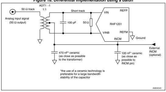
Figure 18. Differential implementation using a balun
