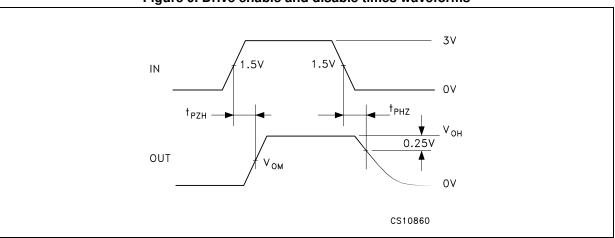
Figure 9. Drive enable and disable times waveforms
