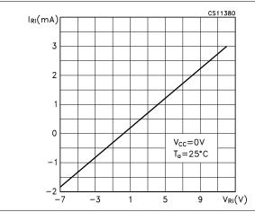
Figure 22. Receiver output current vs output high voltage
