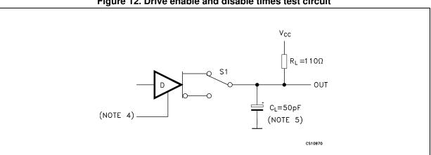
Figure 12. Drive enable and disable times test circuit
