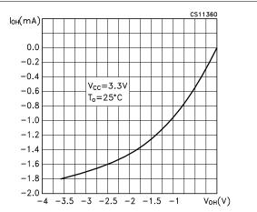
Figure 24. High level driver output capability
