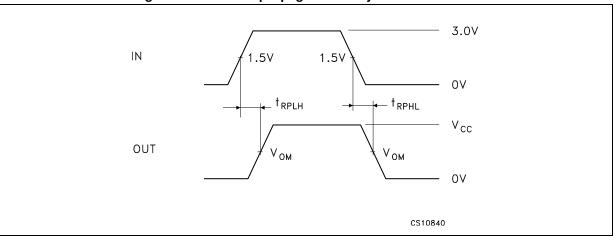
Figure 15. Receiver propagation delay time waveforms
