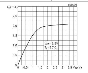
Figure 23. Low level driver output capability
