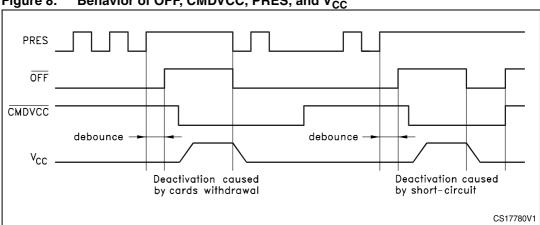
Figure 8. Behavior of OFF, CMDVCC, PRES, and V<sub>CC</sub>
