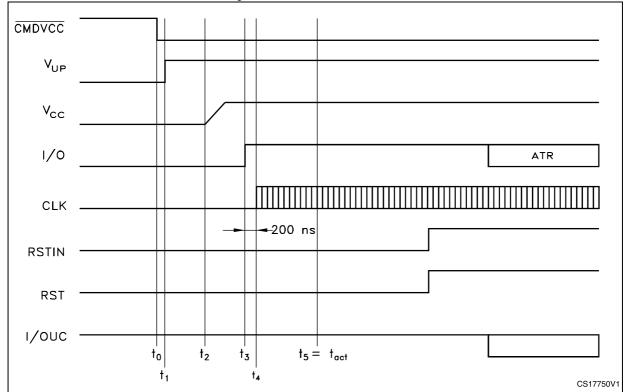
Figure 6. Activation sequence at t<sub>3</sub>
