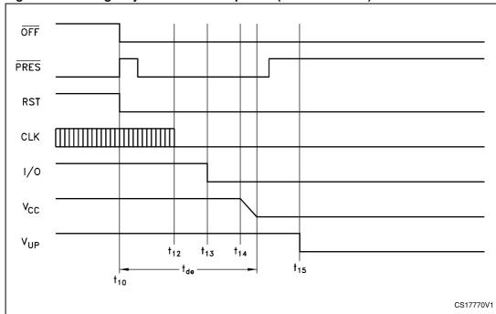
Figure 9. Emergency deactivation sequence (card extraction)
