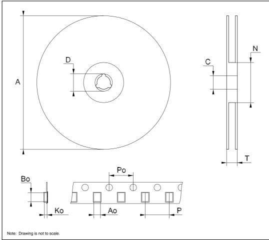
Figure 16. TSSOP-28 tape and reel schematic
