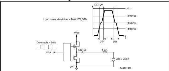
Figure 4. Current dead time test circuit
