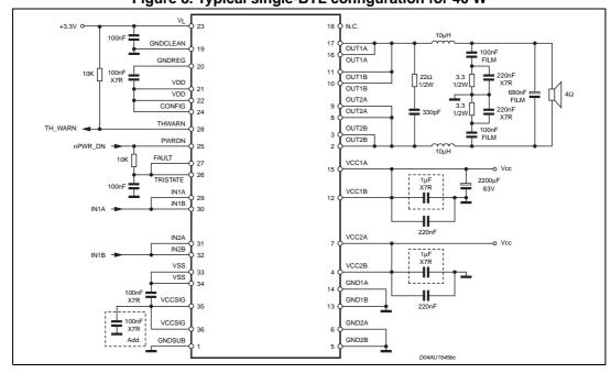
Figure 8. Typical single-BTL configuration for 40 W
