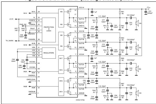
Figure 1. STA515W circuit for quad single-ended amplifiers
