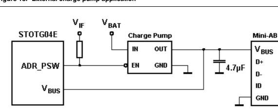
Figure 13. External charge pump application
