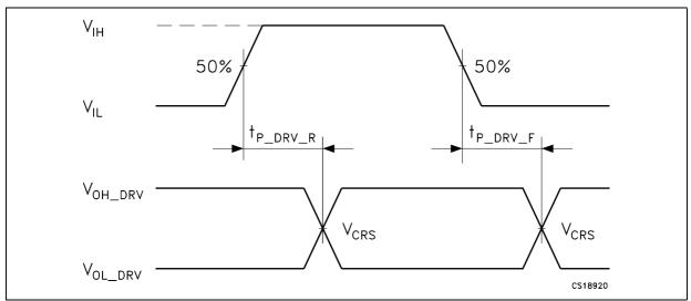
Figure 7. Differential receiver propagation delay
