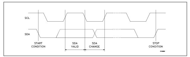
**Start condition** is identified by a falling edge of the SDA signal while the SCL is stable at high level. The start condition must precede any data transfer on the bus.
