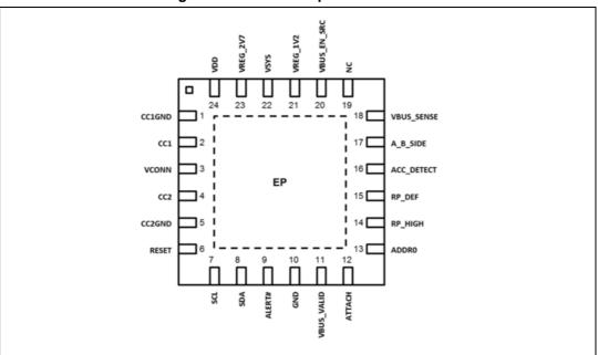
Figure 2. STUSB1700 pin connections
