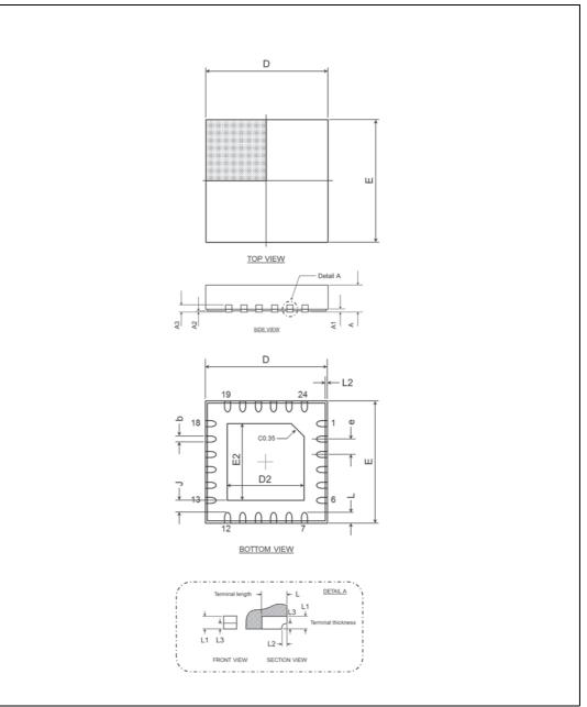
Figure 9. QFN-24 EP 4x4 mm Wet Flk package outline
