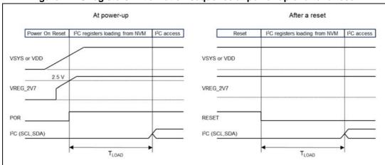
Figure 7. I<sup>2</sup>C registers initialization sequence at power-up or after a reset
