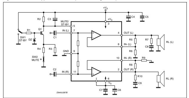
Figure 4. Test and Application Circuit (Stereo Configuration)
