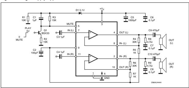
**ELECTRICAL CHARACTERISTCS** (Refer to the test circuit  $V_S = \pm 16V$ ;  $R_L = 8\Omega$ ;  $R_S = 50\Omega$ ;  $G_V = 30dB$ , f = 1KHz;  $T_{amb} = 25^{\circ}C$ , unless otherwise specified)
