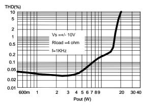
Figure 9. Distortion vs Output Power
