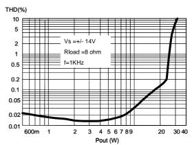
Figure 8. Distortion vs Output Power
