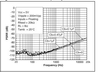
Figure 29. PSRR vs. frequency
