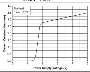
Figure 4. Current consumption vs. standby voltage
