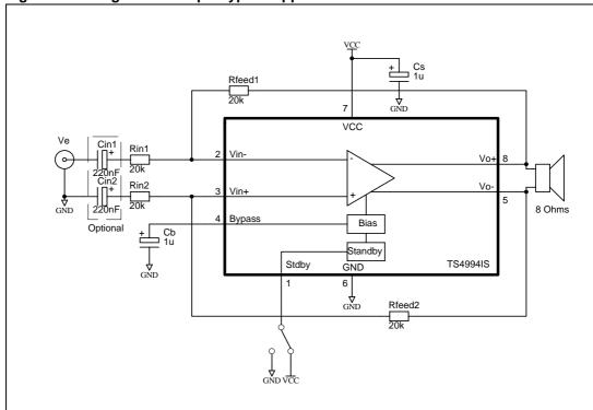
Figure 79. Single-ended input typical application
