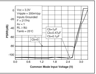
Figure 33. PSRR vs. common mode input voltage
