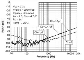
Figure 27. PSRR vs. frequency
