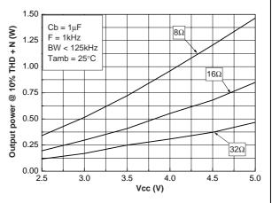
Figure 13. Output power vs. load resistance
