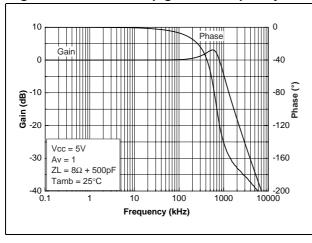
Figure 20. Closed loop gain vs. frequency
