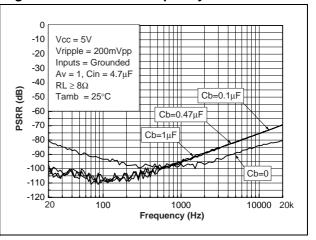
Figure 23. PSRR vs. frequency
