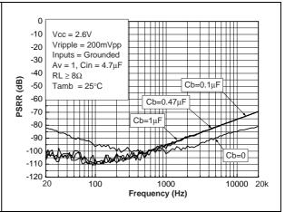
Figure 25. PSRR vs. frequency
