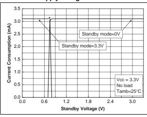
Figure 6. Current consumption vs. standby voltage
