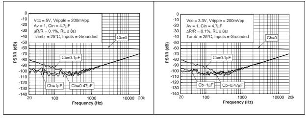
Figure 72. PSRR vs. frequency (worst case conditions)
