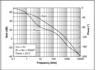
Figure 17. Open loop gain vs. frequency
