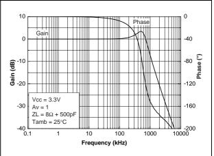
Figure 21. Closed loop gain vs. frequency
