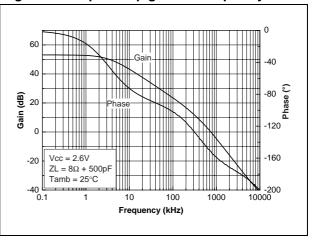
Figure 19. Closed loop gain vs. frequency
