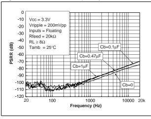
Figure 30. PSRR vs. frequency
