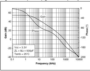
Figure 18. Open loop gain vs. frequency
