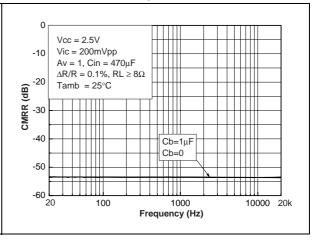
Figure 77 and Figure 78 show CMRR versus frequency for a typical application with a random selection of four  $\Delta$ R/R values with a 0.1% tolerance.
