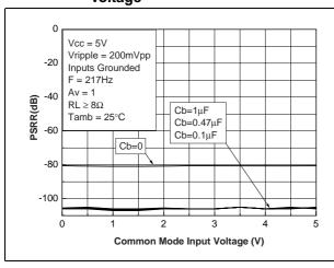
Figure 32. PSRR vs. common mode input voltage
