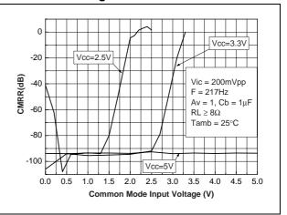
Figure 41. CMRR vs. common mode input voltage
