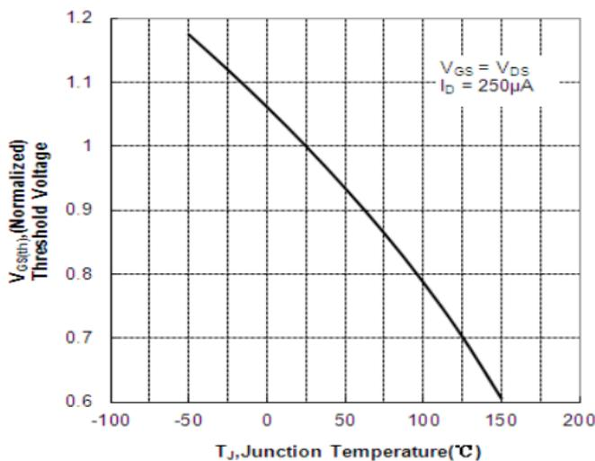
Figure 10 Typical Theshold Voltage vs Junction Temperature
