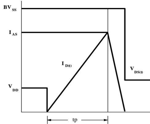
**4) Unclamped Inductive Switching Test Circuit & Waveforms**
