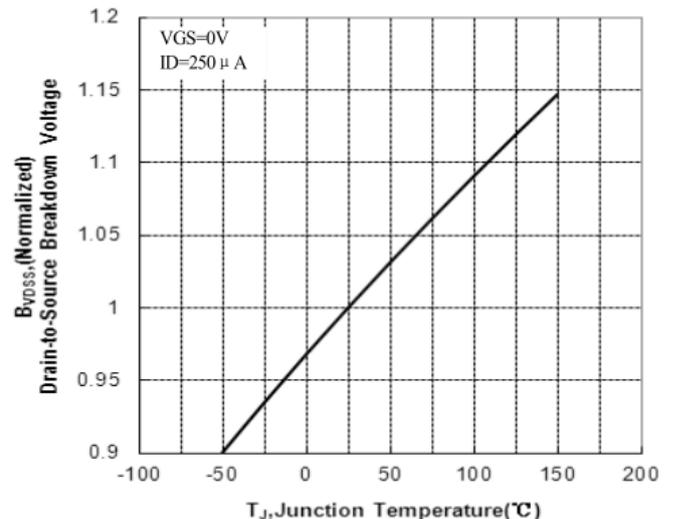
Figure 11 Typical Breakdown Voltage vs Junction Temperature
