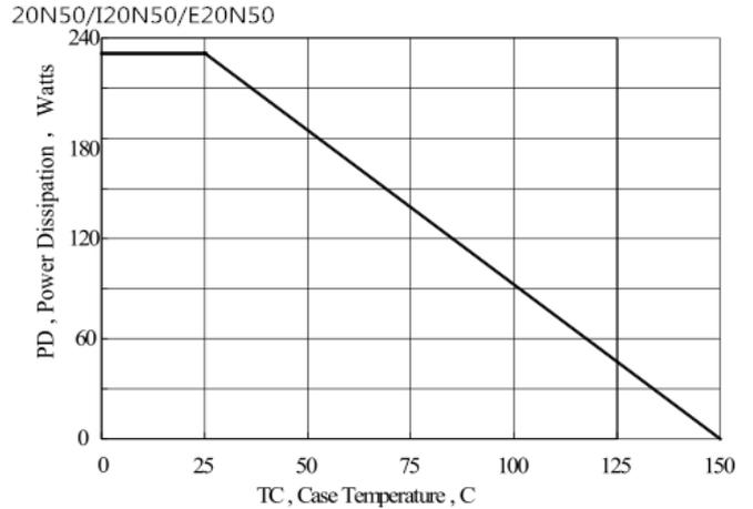
Figure 2 Maximum Power Dissipation vs Case Temperature
