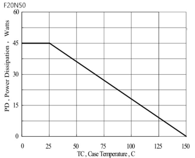
Figure 15 Maximum Power Dissipation vs Case Temperature
