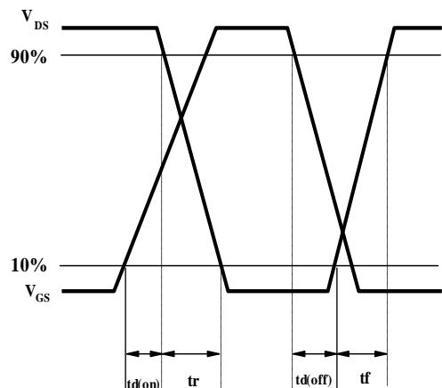
2) Resistive Switching Test Circuit & Waveforms
