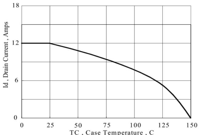
Figure 3 Maximum Continuous Drain Current vs Case Temperat
