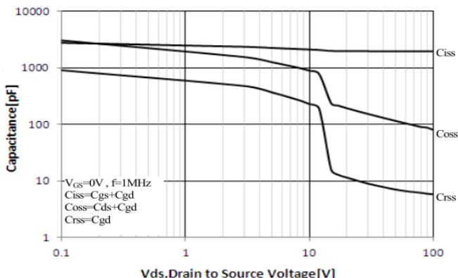
Figure 12 Typical Capacitance vs Drain to Source Voltage
