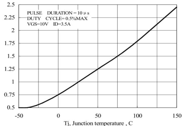
Figure 9 Typical Drian to Source on Resistance vs Junction Temperature
