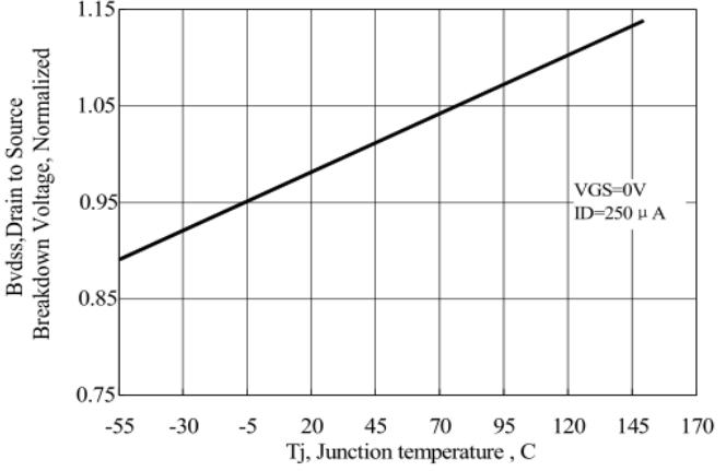
Figure 11 Typical Breakdown Voltage vs Junction Temperature
