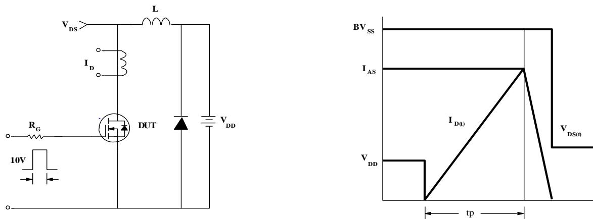
4) Unclamped Inductive Switching Test Circuit & Waveforms
