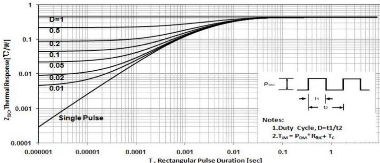
Figure 5 Maximum Effective Thermal Impedance . Junction to Case
