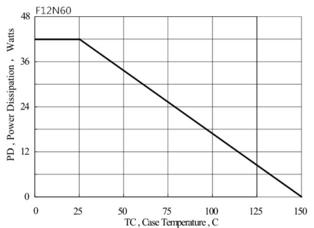
Figure 15 Maximum Power Dissipation vs Case Temperature
