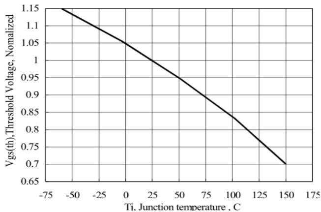
Figure 10 Typical Threshold Voltage vs Junction Temperature
