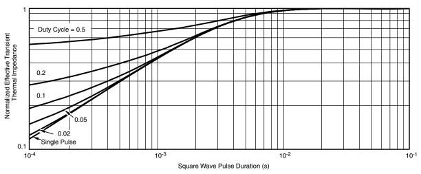
Normalized Thermal Transient Impedance, Junction-to-Case
