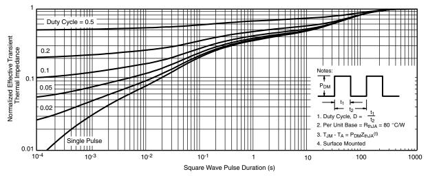
Normalized Thermal Transient Impedance, Junction-to-Ambient
