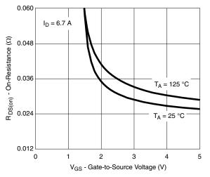
On-Resistance vs. Gate-to-Source Voltage
