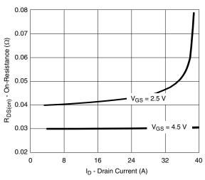
On-Resistance vs. Drain Current and Gate Voltage
