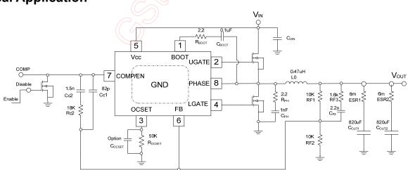
Figure 1 Typical Application of GS7256
