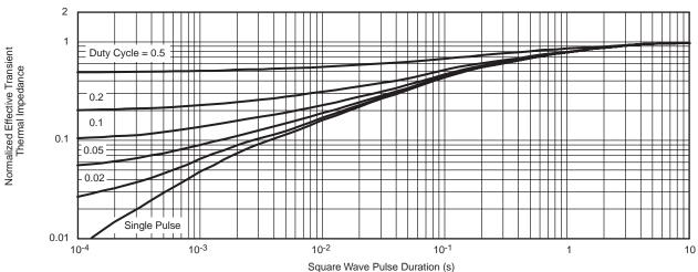
Normalized Thermal Transient Impedance, Junction-to-Foot
