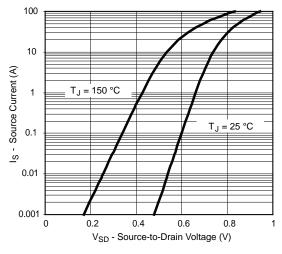
Forward Diode Voltage vs. Temperature
