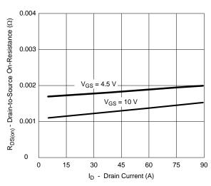
R<sub>DS(on)</sub> vs. Drain Current
