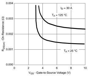
$R_{DS(on)}$  vs.  $V_{GS}$  vs. Temperature
