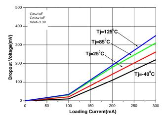
Figure 14. Dropout Voltage vs. Loading Current
