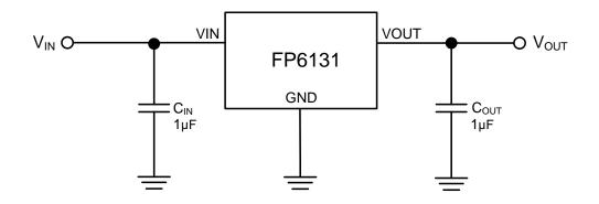
Figure 2. Typical Application Circuit of FP6131
