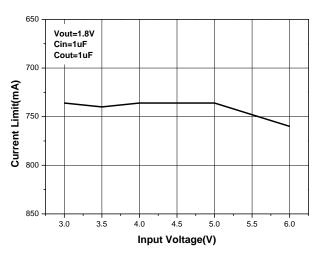
Figure 6. Current limit vs. Input Voltage
