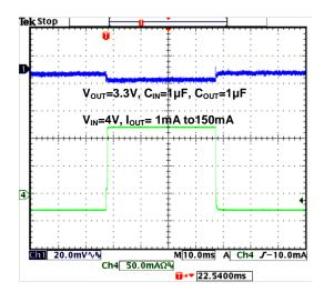
Figure 15. Load Transition Response
