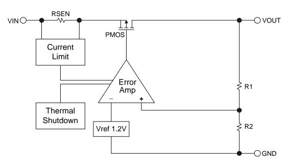
Figure 3. Block Diagram of FP6131
