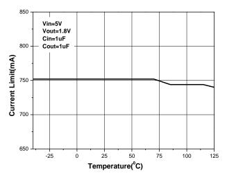
Figure 8. Current limit vs. Temperature
