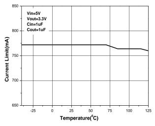
Figure 9. Current limit vs. Temperature
