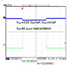
Figure 16. Load Transition Response
