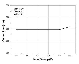
Figure 7. Current Limit vs. Input Voltage
