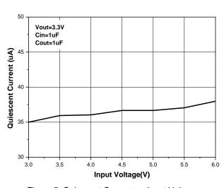
Figure 5. Quiescent Current vs. Input Voltage
