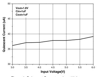
Figure 4. Quiescent Current vs. Input Voltage
