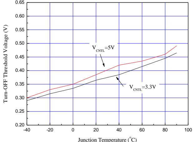
Figure 5. Turn-Off Threshold Voltage vs. Junction Temperature
