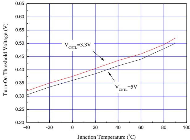
Figure 4. Turn-On Threshold Voltage vs. Junction Temperature
