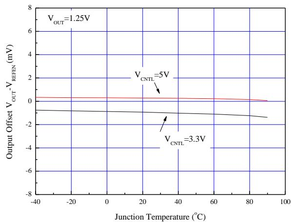
Figure 6. Output offset (V<sub>OUT</sub>-V<sub>REFEN</sub>) vs. Junction Temperature
