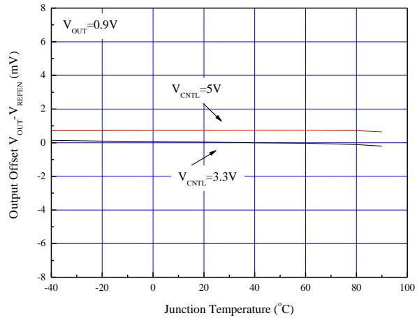
Figure 7. Output offset (V<sub>OUT</sub>-V<sub>REFEN</sub>) vs. Junction Temperature
